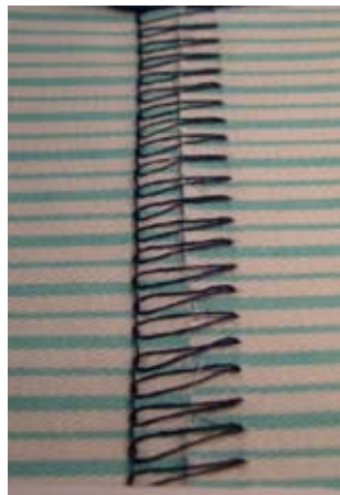
4-thread, 5/32" wide, 17 stitches per inch Photo: Merrow Sewing Machine Company
