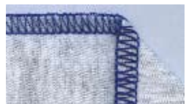
4-thread, 5/32" wide, 17 stitches per inch, Photo: Merrow
