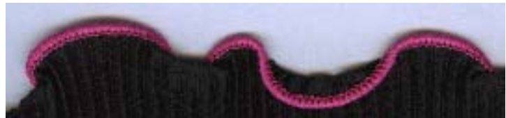
2-thread, 1/8" wide, 20 stitches per inch, with differential feed: Photo: Merrow
